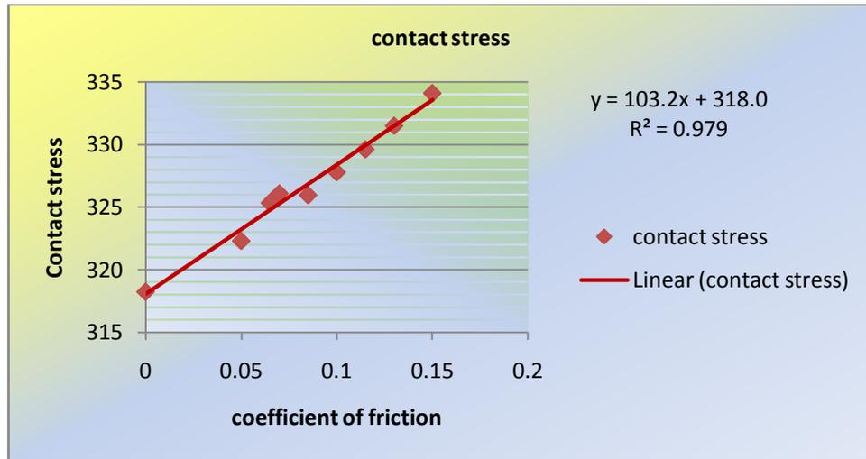
Fig.6 effect of coefficient of friction on contact stress of stage 1
