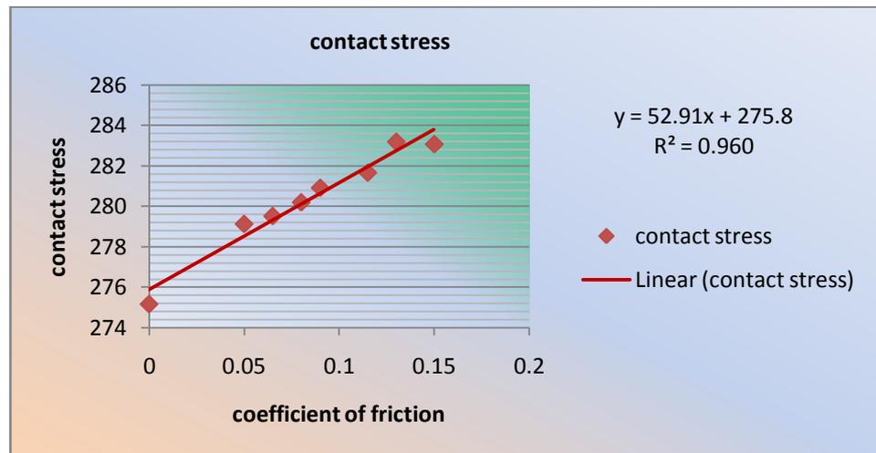
Fig.7 effect of coefficient of friction on contact stress of stage 2
