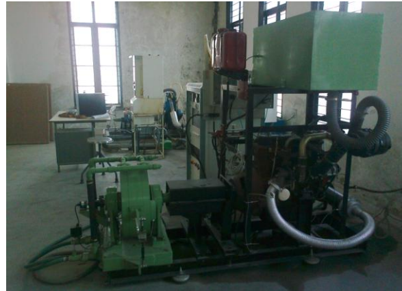
Fig.4 Photograph of multi-cylinder C.I. engine test Rig
